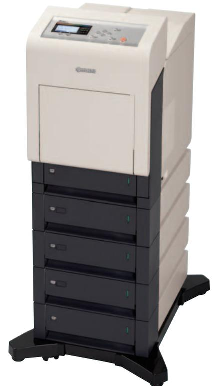
FS-C5400DN configuration shown with four (4) optional paper feeders (PF-500 and/or PF-510) and caster kit (CA-500).
